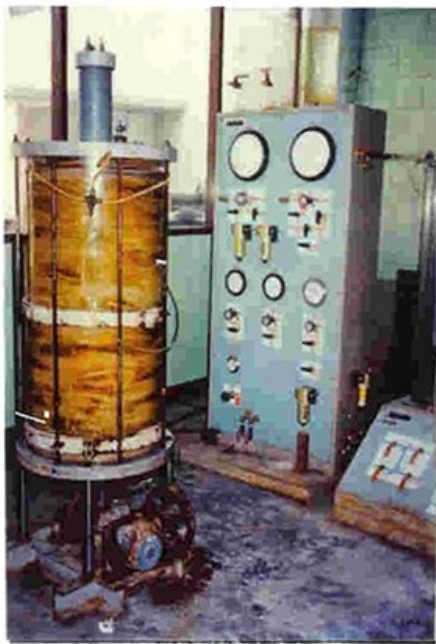
Fig. A-16 Large Consolidometer with Central Drainage
