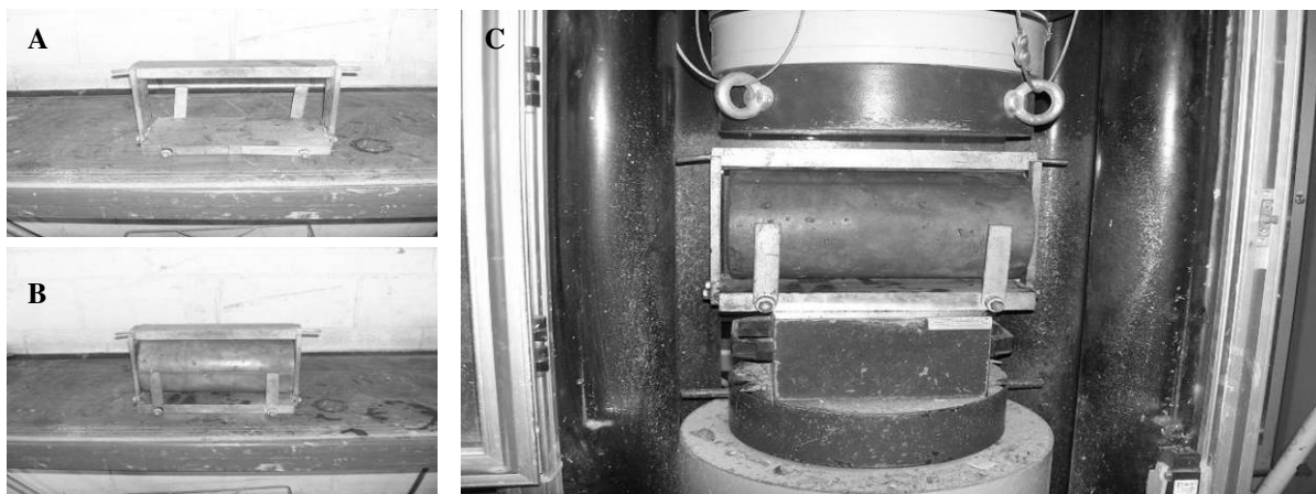
Figure 5: Jig without a test cylinder (A), Jig with a test cylinder (B) and the jig with a test cylinder inside the hydraulic compression machine (C).
