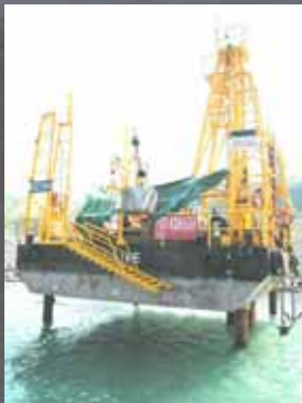
Jack-up rig with legs deployed and raised above water level
