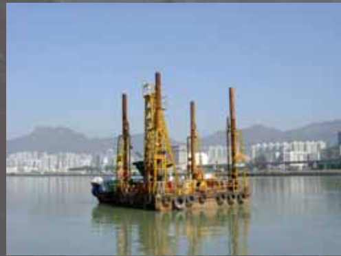
Jack-up barge being floated into position
