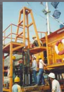
Cone Penetration Test (CPT) reaction frame
