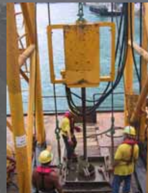
Vibrocore tube and vibrator
