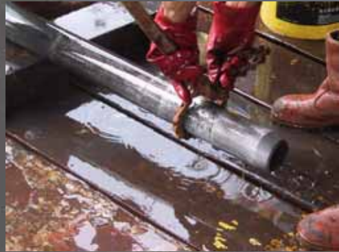
Removal of cutting shoe
