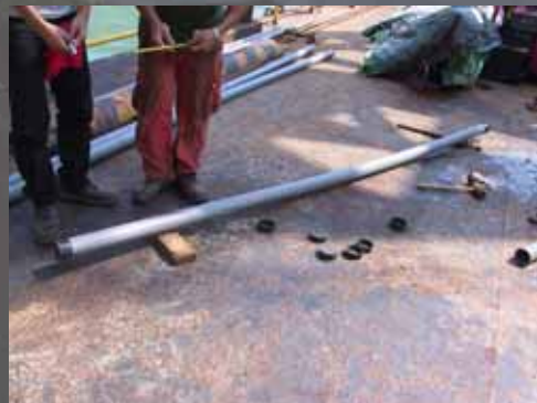
Vibrocore sample in PVC liner - 6m per run
