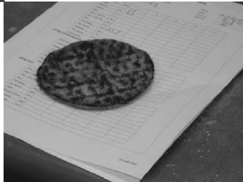
GCL Sample ready for Testing
