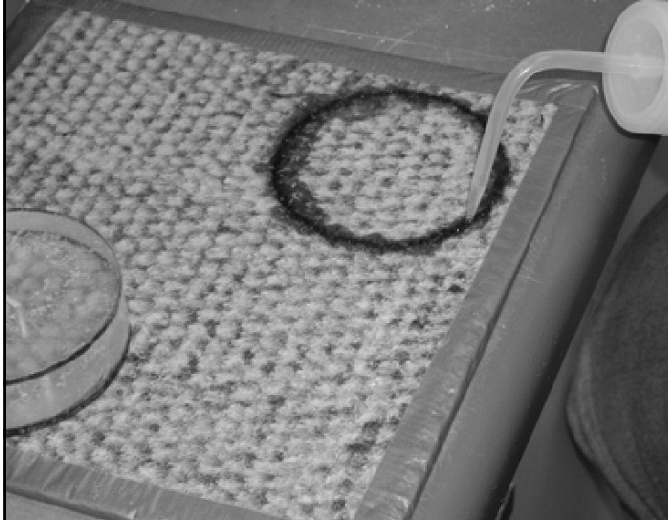
Cutting a GCL sample from a 30 cm 2 square specimen
