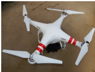
(a) UAV (PHANTOM2) with digital camera
