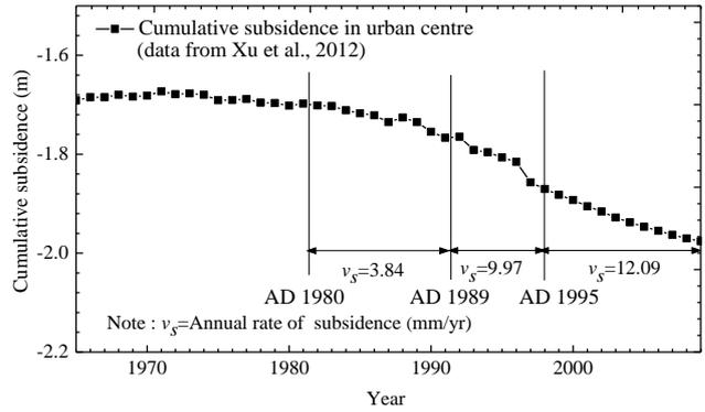
Figure 3 Cumulative subsidence from 1965 to 2010 in Shanghai
