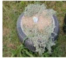
Filling: Tire chips + soils Placement: Two layers (vertical)
