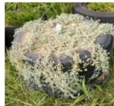
Filling: Tire chips + soils Placement: Two layers (vertical)
