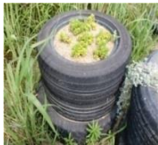
Filling: Soils Placement: Three layers (vertical)
