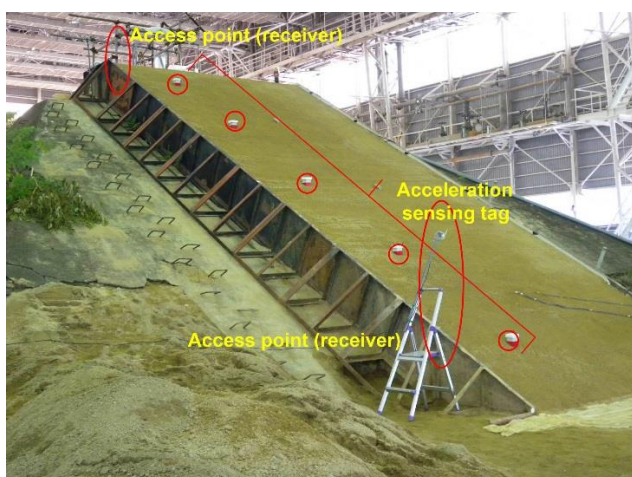
Figure 23 Outline of model tests on slope failure caused by rainfall
