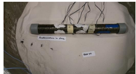
Partially completed model with instrumented pipe
