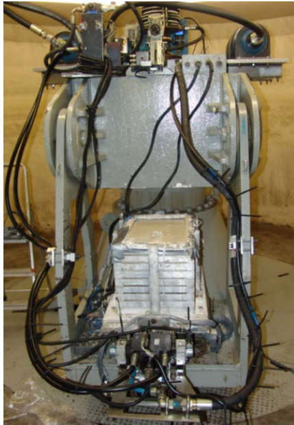
Centrifuge Model Setup with Laminar Box Containing Soft Clay and Embedded Pile Group System
