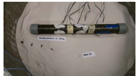
Partially Completed Model with Instrumented Pipe
