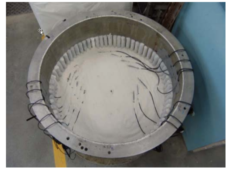
Partially Completed Centrifuge Blast Test Model during Sensor Placements
