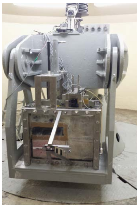
Fig. 2. Centrifuge modelling of tunnels with improved soil surround and heading.
