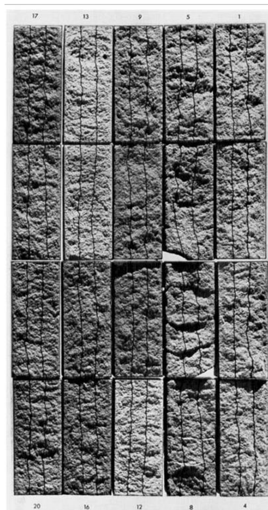
Fig. 2.11 Rock surface roughness profiles obtained from a classic photogrammetric method (Wickens & Barton, 1971)
