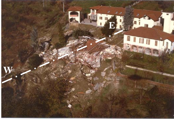
Figure 8. Aerial photograph showing the San Raffaele Cimena landslide site. Also shown is the trace of the E-W cross section given in Figure 9.
