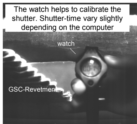
Figure 1- 8: Calibration of the Shutter of the camera
