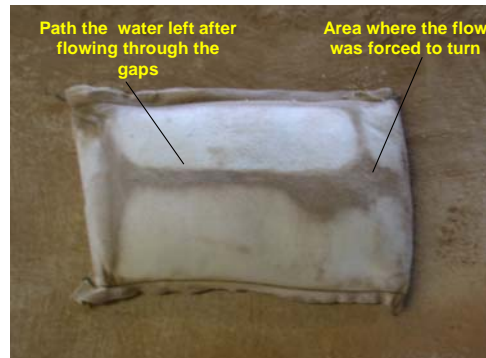
Figure 11: Container after the Permeability Tests (marks of water flow clearly seen)
