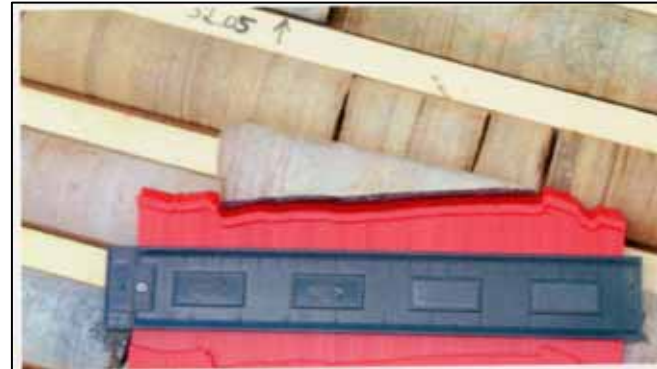
Figure 3. Example of a/L and JRC estimation, set 2 ( JRC \approx 4-6 ).
