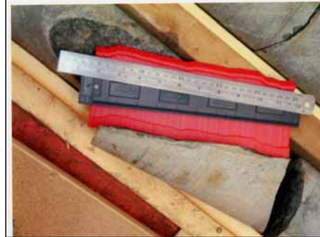
Figure 3. Example of a/L and JRC estimation, set 2 ( JRC \approx 4-6 ).
