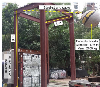
Figure 66. Pendulum impact facility (Ng et al. 2016a)
