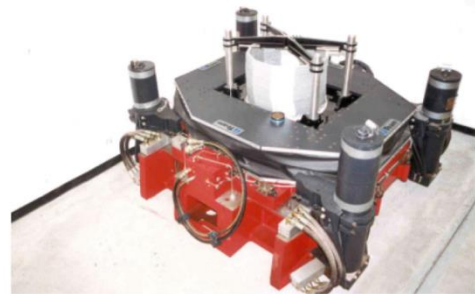
Figure 57. Bi-axial (2D) shaking table (Ng et al. 2004)
