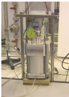
Figure 29. Stress-controlled 1D pressure plate (Ng & Pang 2000)
