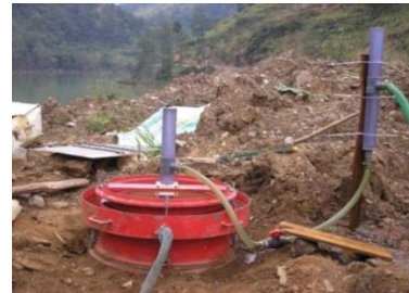
Figure 46. Jet index erodibility testing apparatus (Chang et al. 2011)
