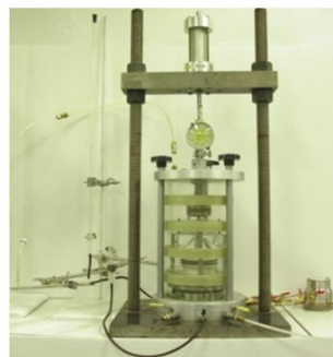
Figure 30. Stress-controlled 3D pressure extractor (Ng et al. 2012)
