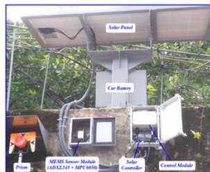
Figure 50. The Smart Soil Particle installed at field
