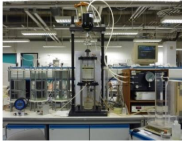
Figure 45. Stress-controlled internal erosion testing apparatus (Chang & Zhang, 2011)
