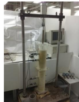
Figure 28. Stress-dependent 1D soil column (Ng & Leung 2011)
