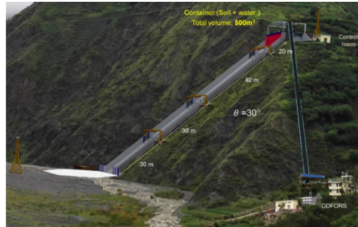
Figure 68. 120-m flume in Kunming, China
