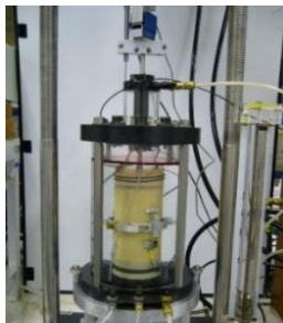
Figure 23. Temperature and suction controlled cyclic triaxial apparatus (Ng & Zhou 2014)
