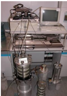
Figure 26. Full suction triaxial apparatus (Ng & Menzies 2007)
