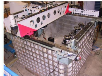
Figure 58. Four-axis (4D) robotic manipulator (Ng et al. 2002)
