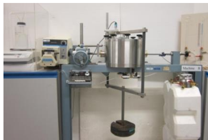
Figure 27. Full-suction direct shear box for unsaturated soil (Ng 2014)
