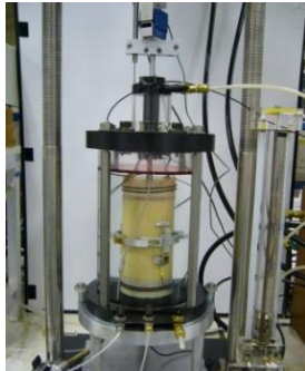
Figure 32. Temperature controlled cyclic triaxial cell (Ng & Zhou 2014)
