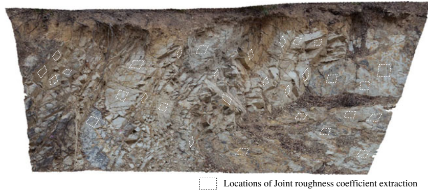
Fig. 7 Roughness profile extraction using the 3D model
