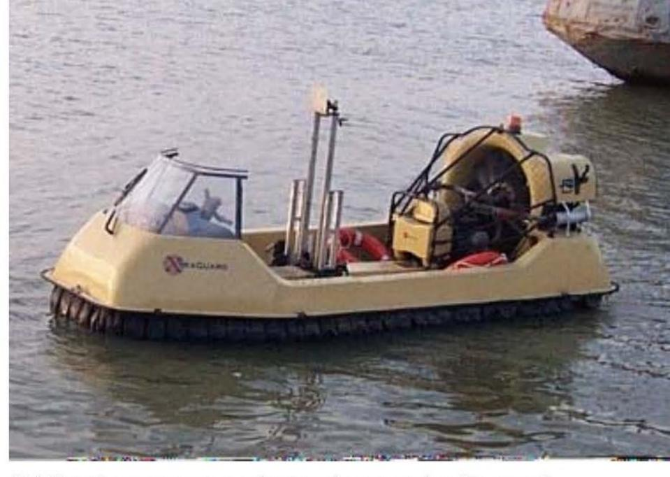
50 kN static penetrometer and rotary rig mounted on Hovercraft
