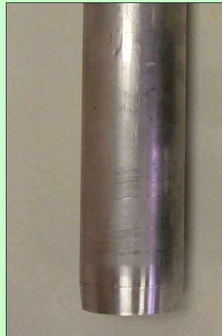
Modified thin-walled (Shelby) tube
