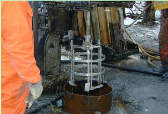
Sampler is lowered into borehole
