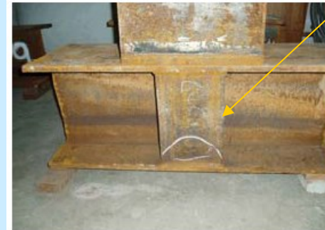
(b) C-channel stiffener (brittle-sway)
