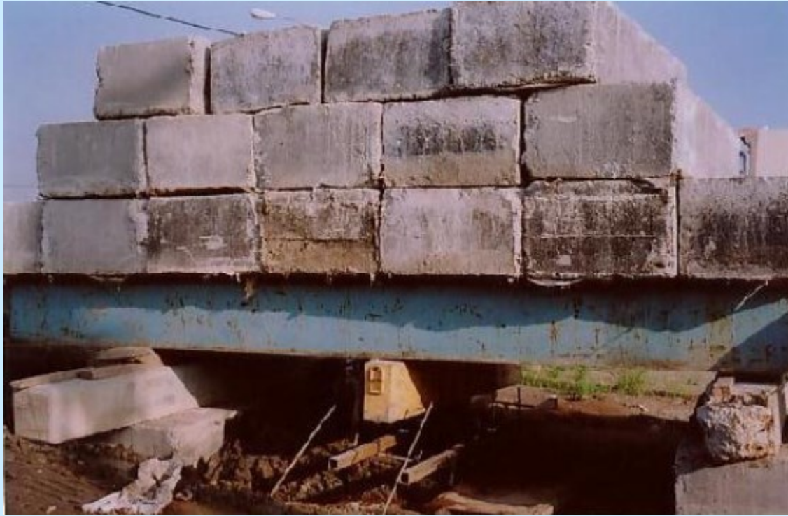
Figure 8.4 Machine in Vietnam and Column Loading test using Concrete block as counter weight
