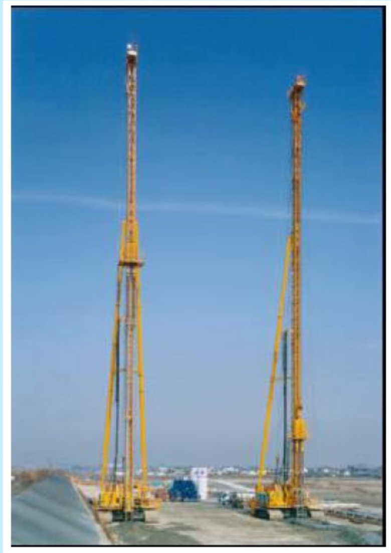
Figure 6.9 Long rod type deep mixing machines
