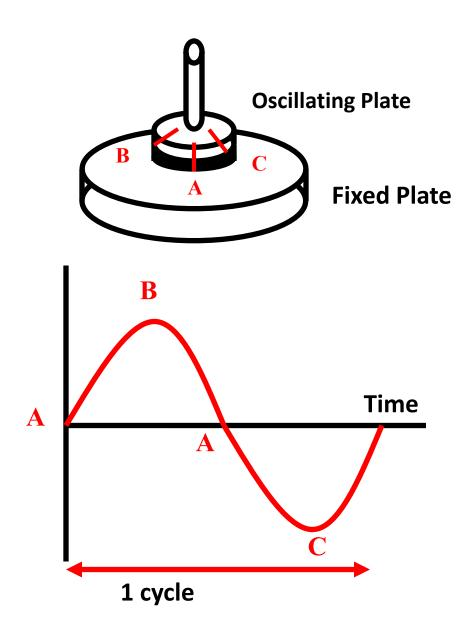
Test operates at 10 rad/sec or 1.59 Hz
