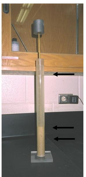
Flocculating Solution Suspended Clay
