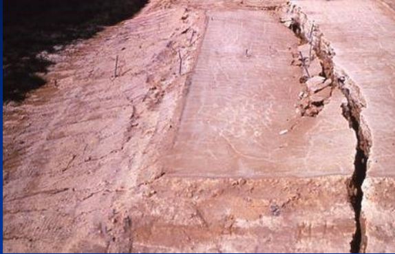
Failure of soft ground under test embankment KL
