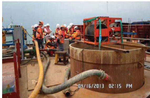
Figure 55. Kodan Verticality Test
