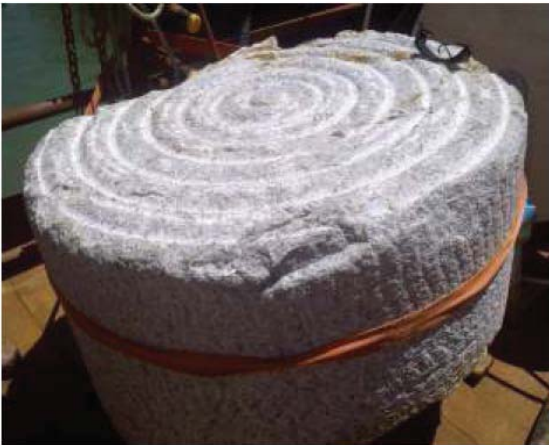
Figure 52. Recovered Granite Rock Core
