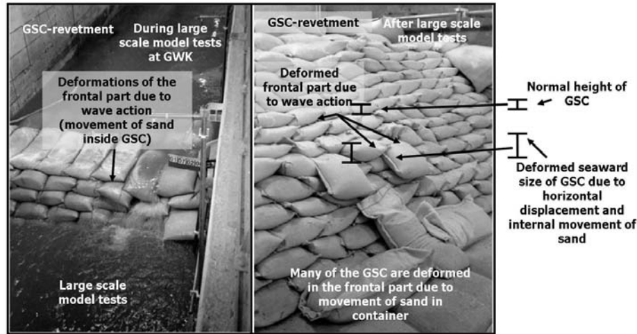
Fig. 21 Observed Failure Mechanisms Under Wave Loads
