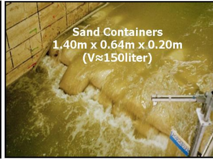
(c) Seaward Dislodgement of Crest Containers in the FZK-Wave Flume.
