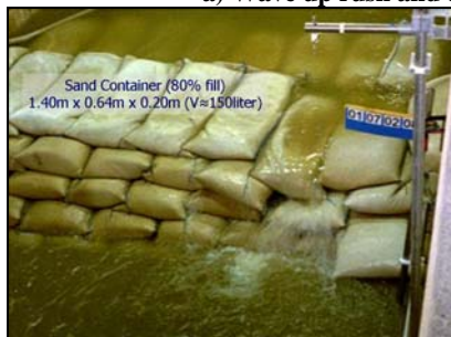
b) Pull out effect in the FZK-large wave flume
