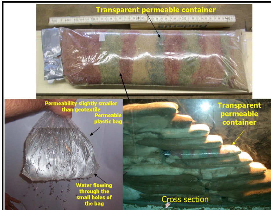
Fig. 25 Permeable Transparent Container for the Investigation of Internal Movement of Sand (Recio and Oumeraci, 2007a)
