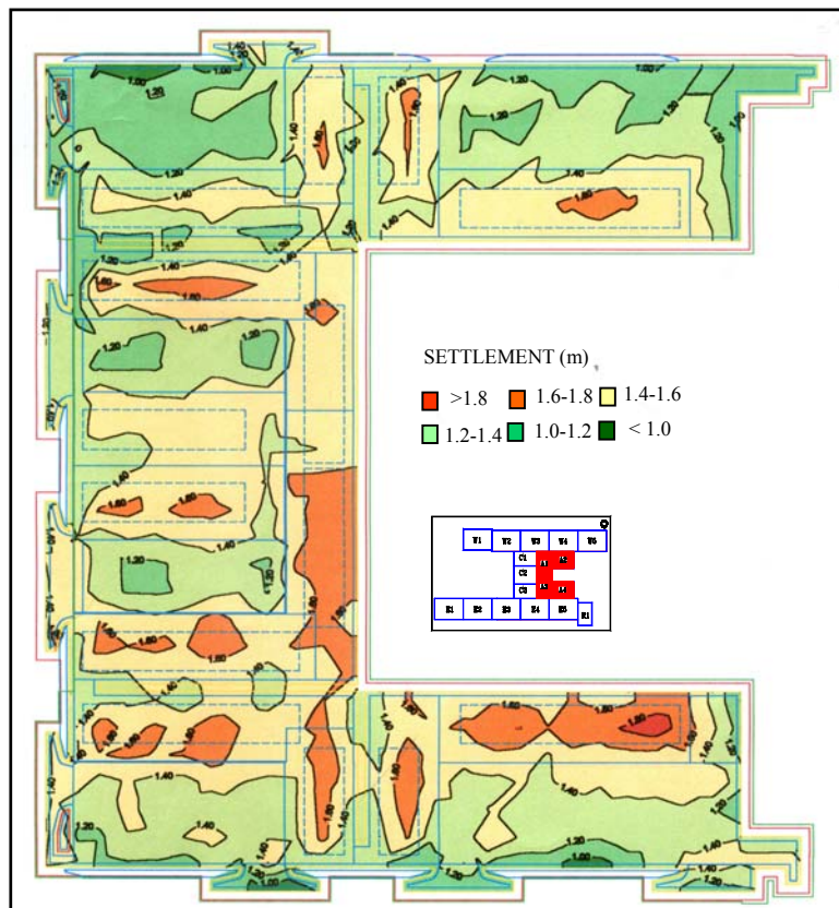
Figure 8 Settlement Contours in the Apron Area
