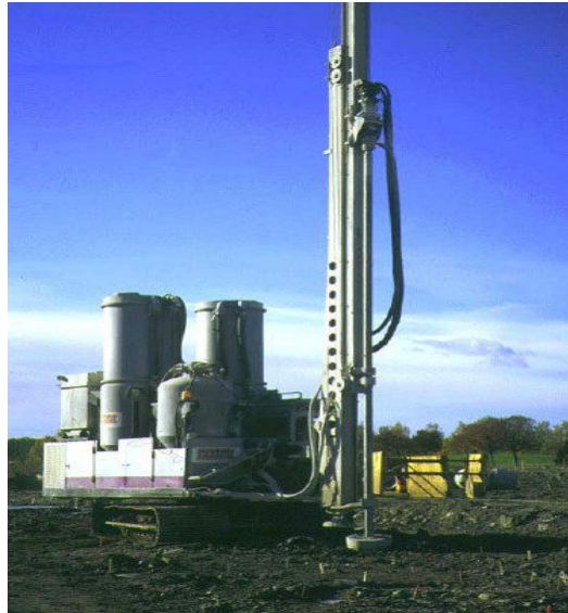
Figure 2.43(c) Deep dry mixing equipment (Massarsch, 2005)
