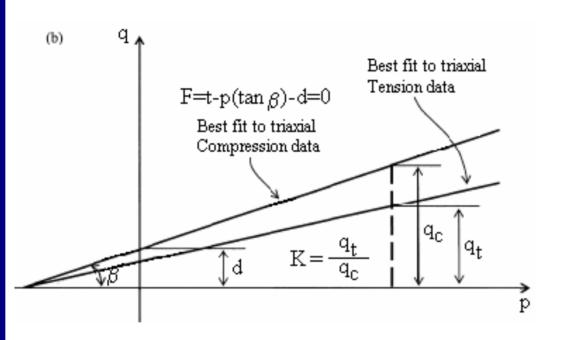
Model parameters obtained from undrained monotonic triaxial tests.
