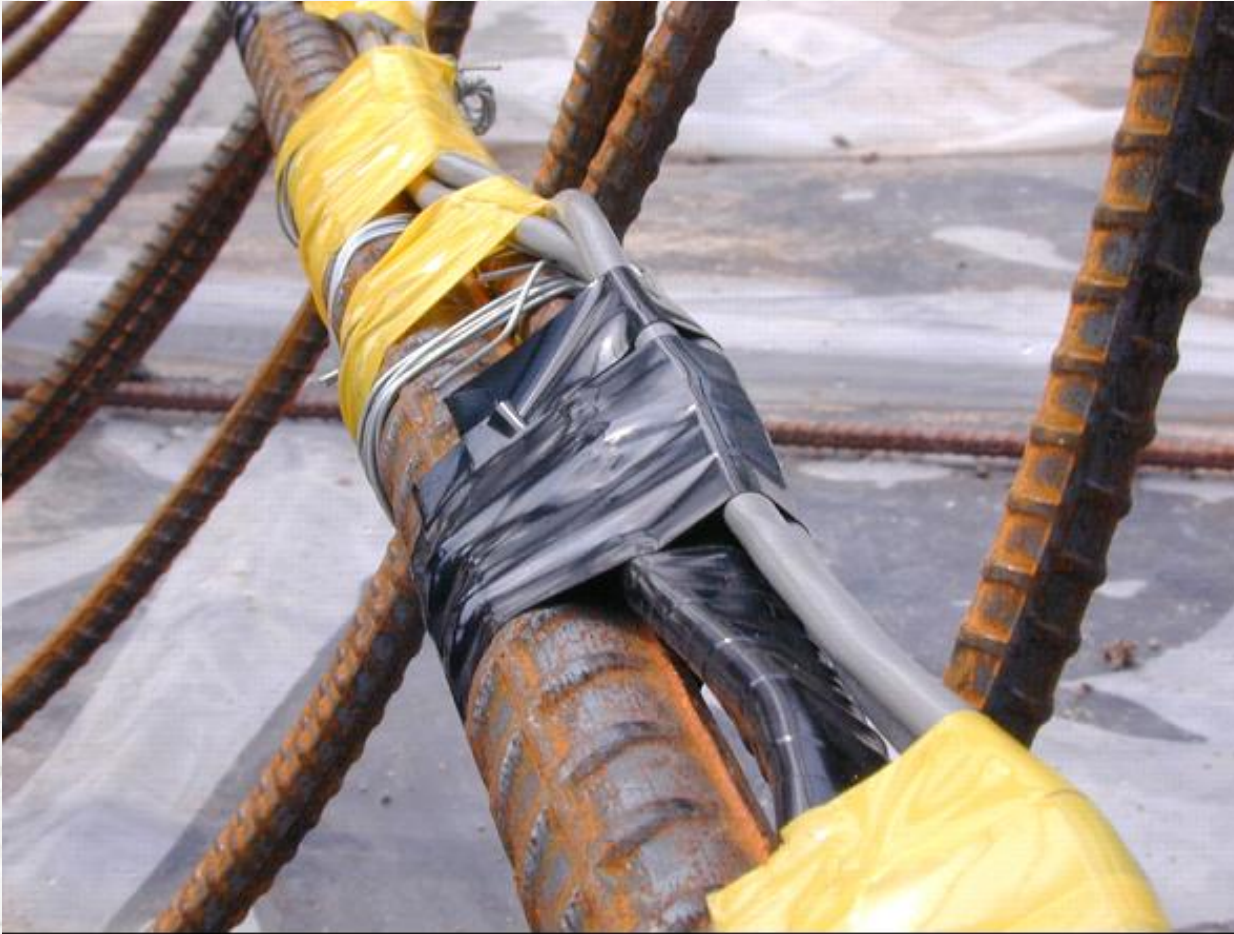
Strain gauges fastened on reinforcement cage of bored piles
