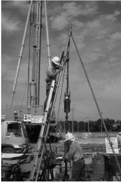
Fig. 1.38 Example of free-fall standard penetration equipment
