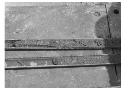
Fig. 1.37 Disturbed soil sample collected by tube
