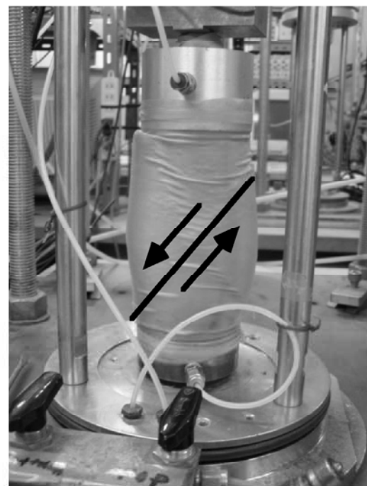
Fig. 1.26 Development of shear failure due to loading of axial stress (Photo by M.Mizuhashi)
