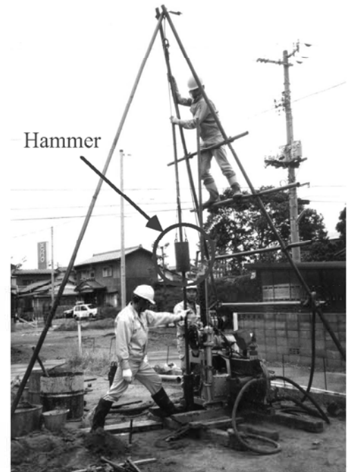
Fig. 1.35 Practice of standard penetration test
