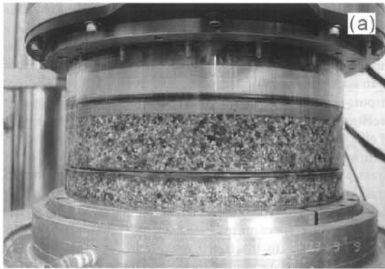
Fig. 15.35 Ring shear test with visual observation of grain behavior (Sassa et al., 2004)
