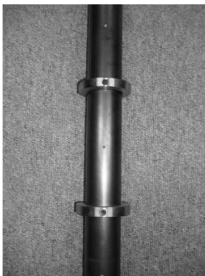
Fig. 13.35 Model of nodular pile for bearing capacity tests
