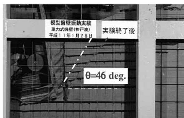
Fig. 12.37 Development of second slip plane after shaking with maximum acceleration = 919 Gal (Photo by K. Watanabe)
