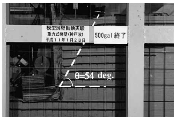
Fig. 12.36 Development of first slip plane after shaking with maximum acceleration = 513 Gal (Photo by K. Watanabe)
