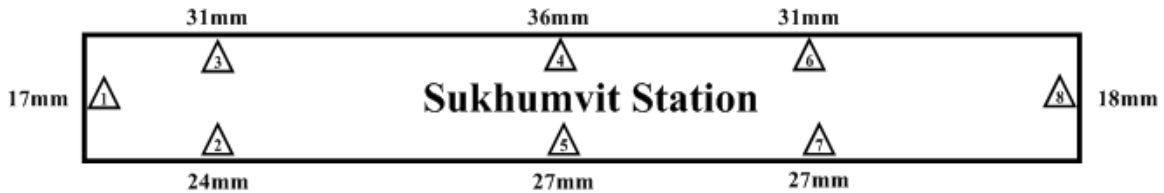
Figure 7.11: Maximum Horizontal Movement of D-Wall (After Stage 4 Excavation)
