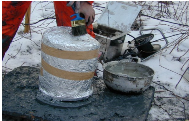
sample initially protected by cling film, tin foil and tape, finally being waxed
