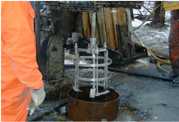
Sampler is lowered into borehole
