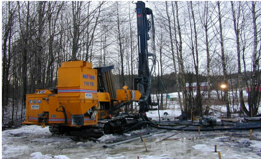
4.2a The drill rig used to operate the block sampler
