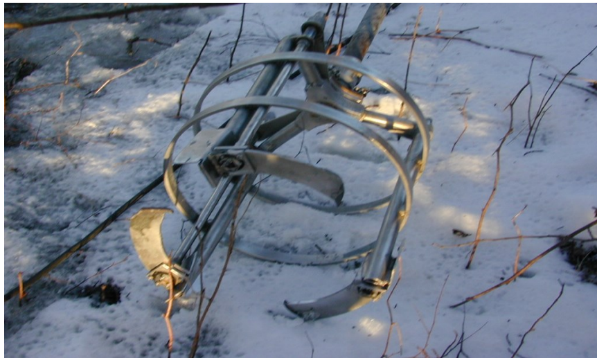
4.2b Close up view of Sherbrooke block sampler
