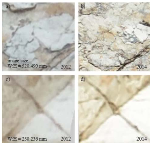
Figure 7 Examples of the 3D image cuts showing the alteration of rock surfaces due to weathering process over two years; shale, section 2 (a, b), sandstone, section 4 (c, d)
