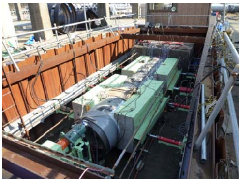
Pipe Jacking (after Le et. al, 2013)
