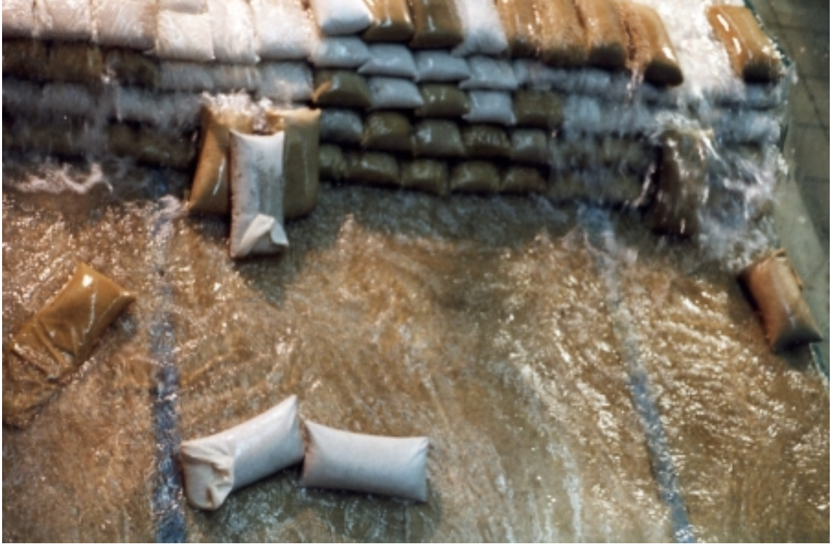
Figure 4: Removed sand containers during small-scale model tests at LWI
