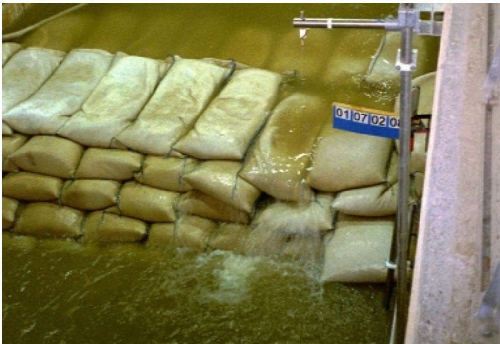
Figure 11: Sand container removed from structure slope
