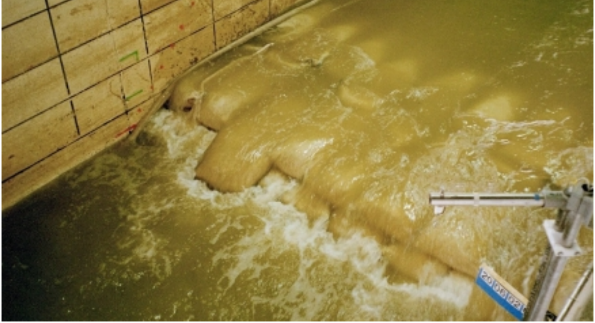
Figure 13: Sand container removed from crest of structure (GWK tests)
