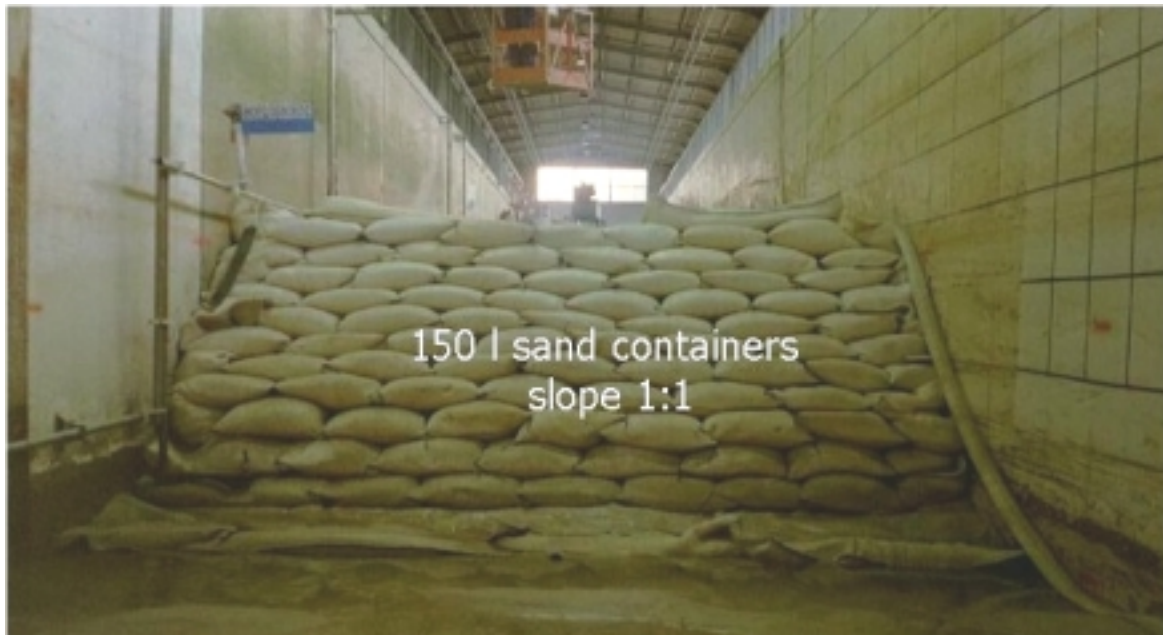
Figure 6: Large-scale model with 150 l sand containers in the Large Wave Flume of Hannover (GWK)
