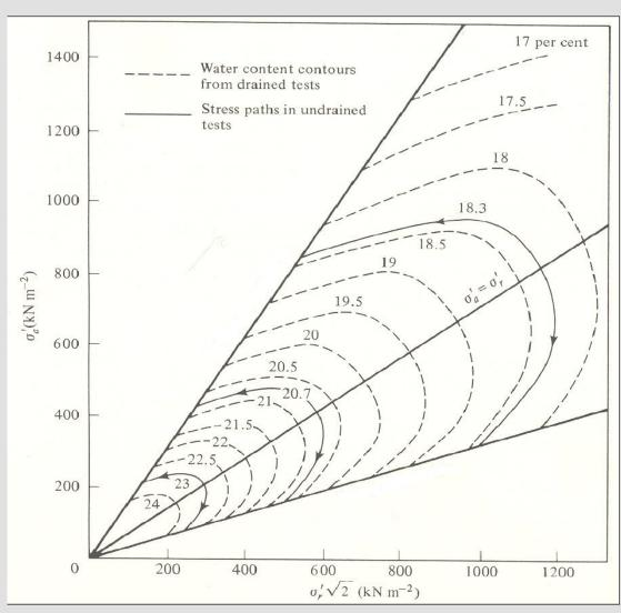
Volumetric yield surface: lines of equal volumetric strains in triaxial test
