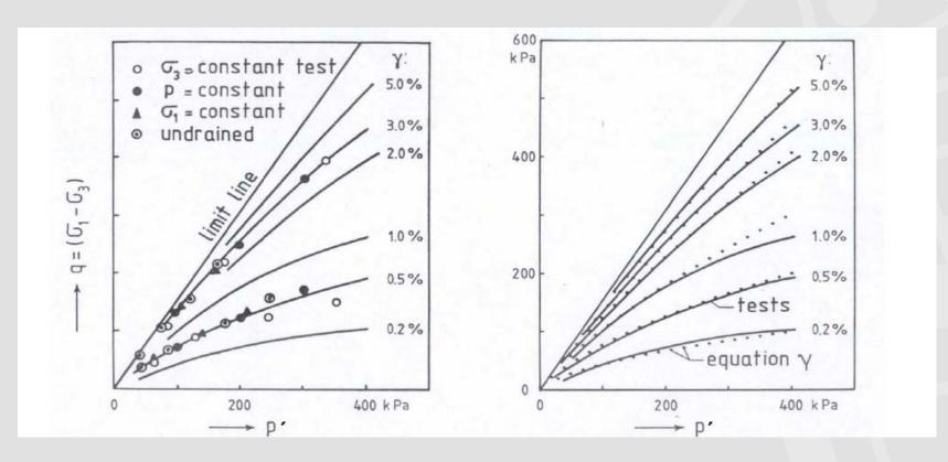
Deviatoric yield surface: lines of equal shear strains in triaxial test
