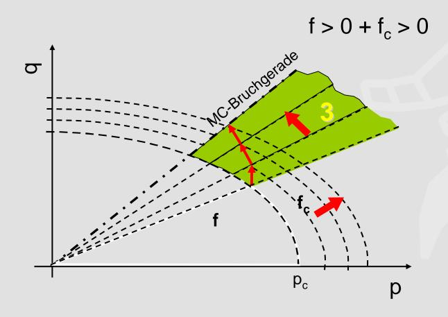
REGION 3 shear hardening and volumetric hardening surfaces active
