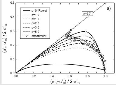
consequence of flow rule in undrained triaxial compression stress path
