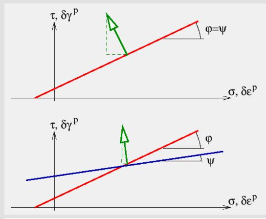
$$f = \frac{1}{2} \left(\sigma'_1 - \sigma'_3\right) + \frac{1}{2} \left(\sigma'_1 + \sigma'_3\right) \sin \varphi' - c' \cos \varphi'$$
