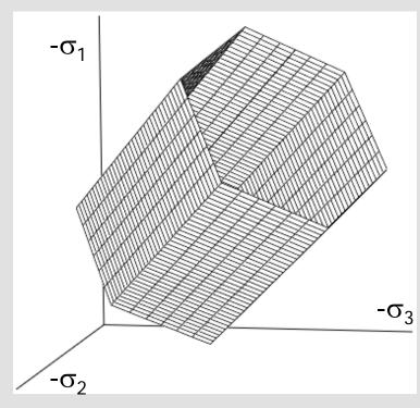
$\psi$  = 0 > no plastic volumetric strains  $\nu$  = 0.495 > negligible elastic volumetric strains
