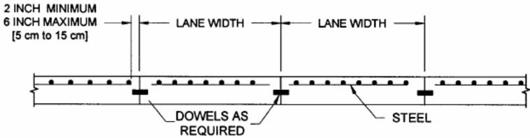
TRANSVERSE CROSS SECTION OF PAVING LANES
