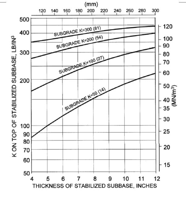
Effect of stabilized subbase on subgrade modulus
