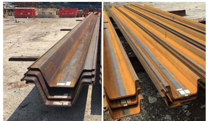
Figure 4 Test piles (Left: Hat-45H-pile, Right: IV-pile)
