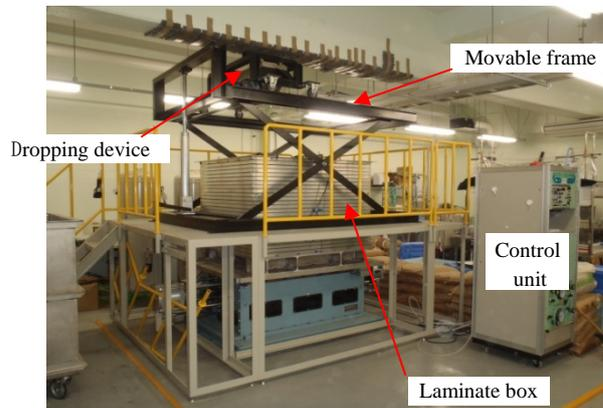
Photo 1 Shaking table test device
