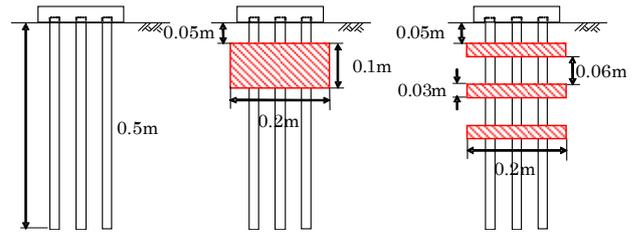
(a) No reinforcement (b) Block reinforcement (c) Multi-layer reinforcement
