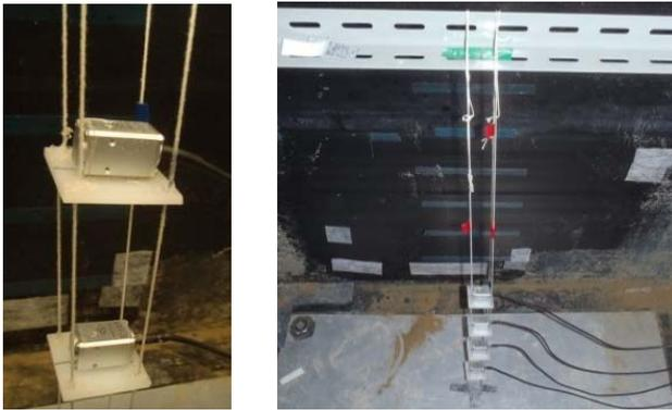
(a) Flexible ring of sockets hosting accelerometers (b) Stiff beam hanged on laminate box
