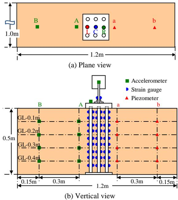
Figure 1 Layout of group-pile foundation and measuring devices in shaking table tests
