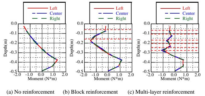
Figure 9 Calculated distribution of bending moments at the time when maximum bending moment happened
