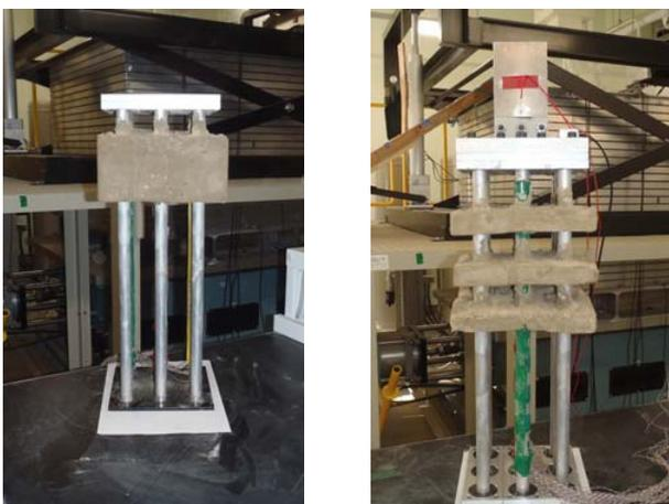
(a) Case 2=Block reinforcement (b) Case 3=Multi-layer reinforcement
