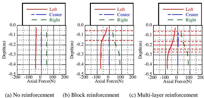
Figure 8 Calculated distribution of axial forces at the time when maximum bending moment happened
