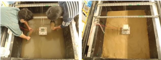
(a) Preparation of saturated ground with in-water sedimentary method (b) Saturated ground after water was taken away
