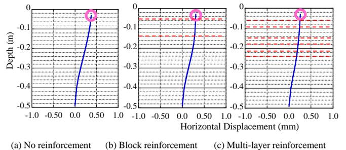
Figure 10 Calculated distribution of horizontal displacement at the time when maximum bending moment happened
