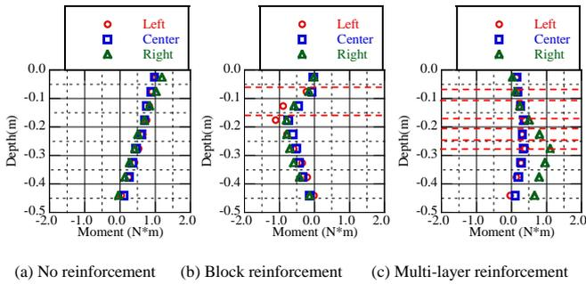
Figure 7 Measured distribution of bending moments at the time when maximum bending moment happened
