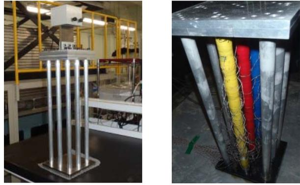
(a) Model 9-pile foundation (b) Piles stuck with strain gauges and covered with water-proof tape
