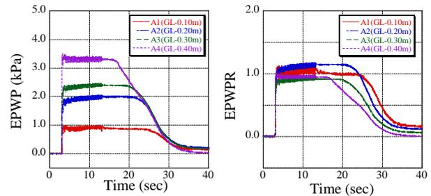
Figure 5 Measured EPWP at different depth in Case 1
