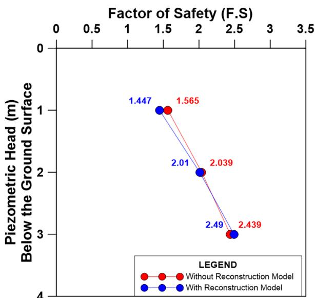
Figure 9 Comparison of simulated FS between reconstructed and non-reconstructed models
