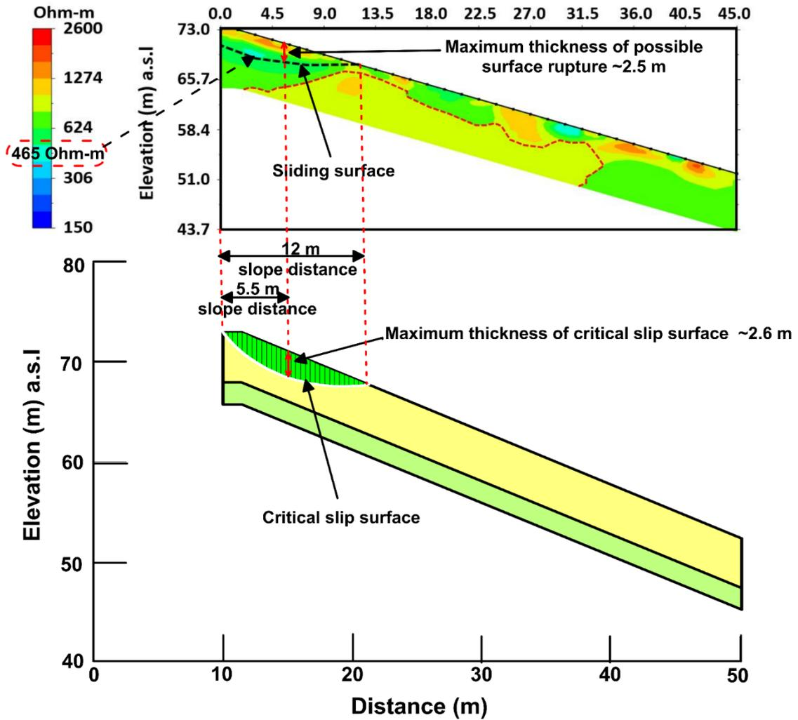
Figure 6 Sliding surface and thickness of sliding mass from slope stability modelling comparing with 2D-ERI
