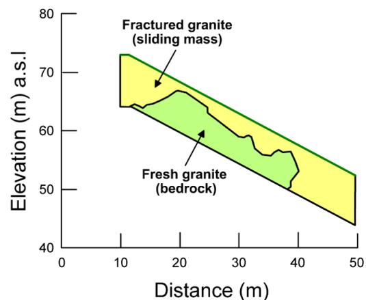
Figure 7 Reconstruction of model geometry using 2D-ERI
