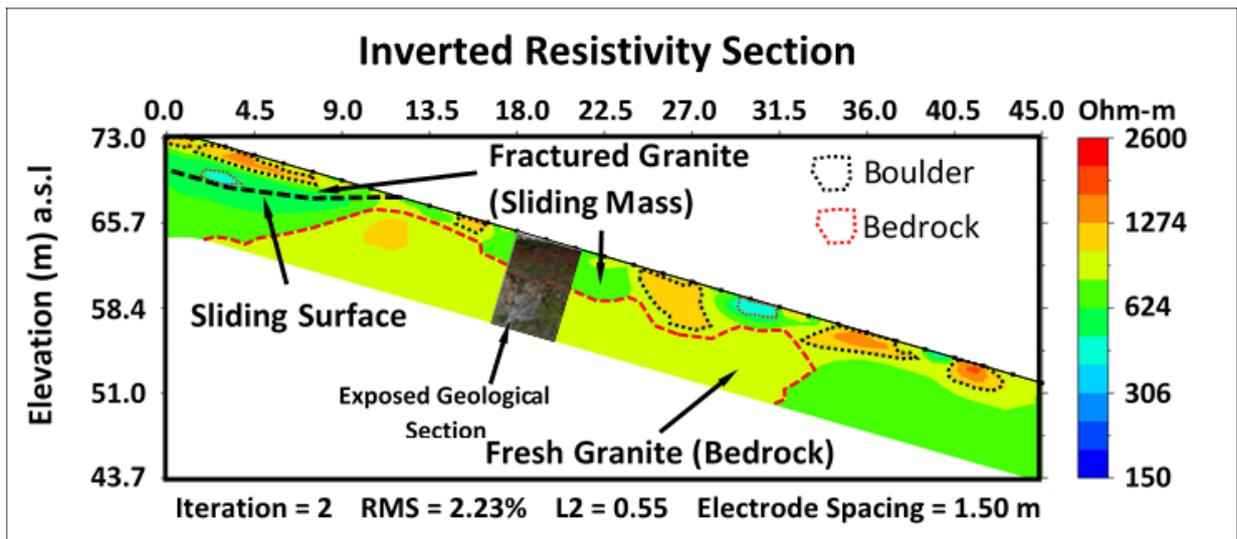
Figure 5 Interpretation of 2D-ERI showing the sliding surface of the susceptible landslide
