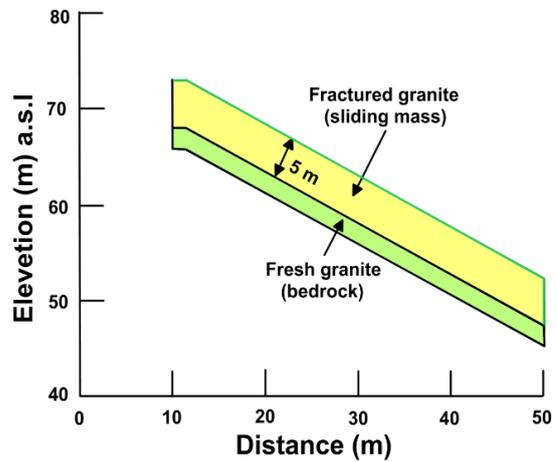
Figure 4 Model geometry for slope stability modelling
