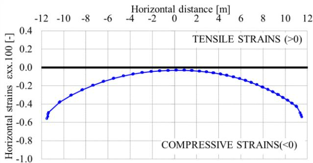
Figure 9 Horizontal strains in the top of the ground improvement block with 5 meters of GI thickness and use of pressure relief wells
