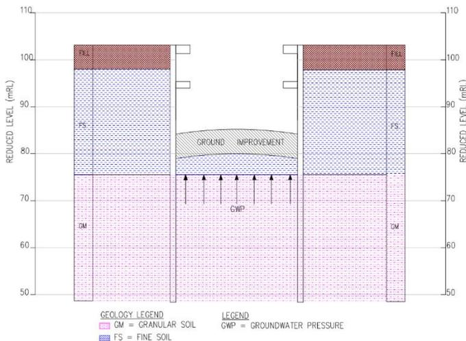
Figure 2 Uplift force below the formation level in a deep excavation
