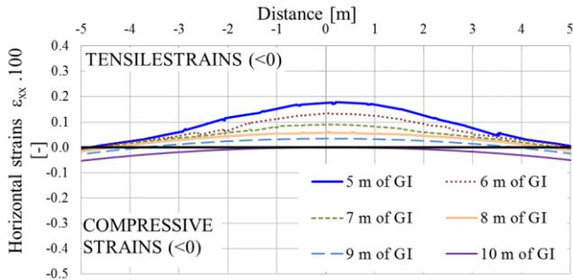
Figure 7 Horizontal strains in the top of the ground improvement layer with different thickness
