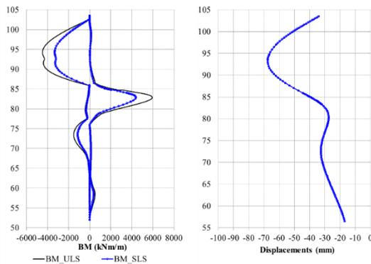
Figure 4 Wall Forces and Displacements of the DWall
