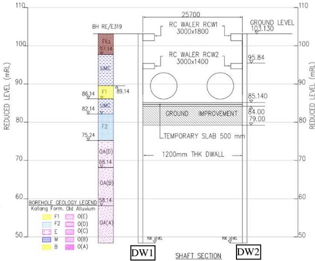
Figure 3 Cross section of the TBM launching shaft with geo profile
