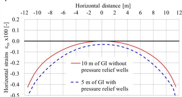
Figure 10 Horizontal strains in the top of the ground improvement block for first and second alternative
