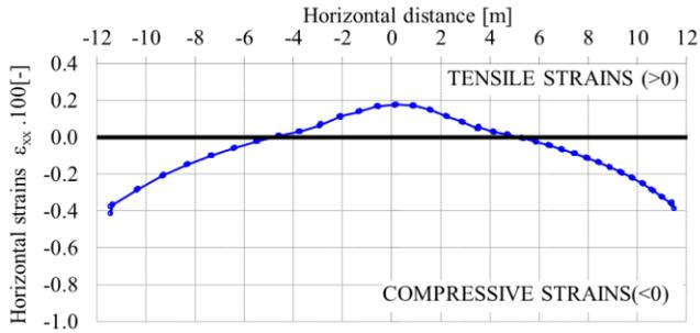
Figure 6 Horizontal strains in the top of the ground improvement block with 5 meters of GI thickness
