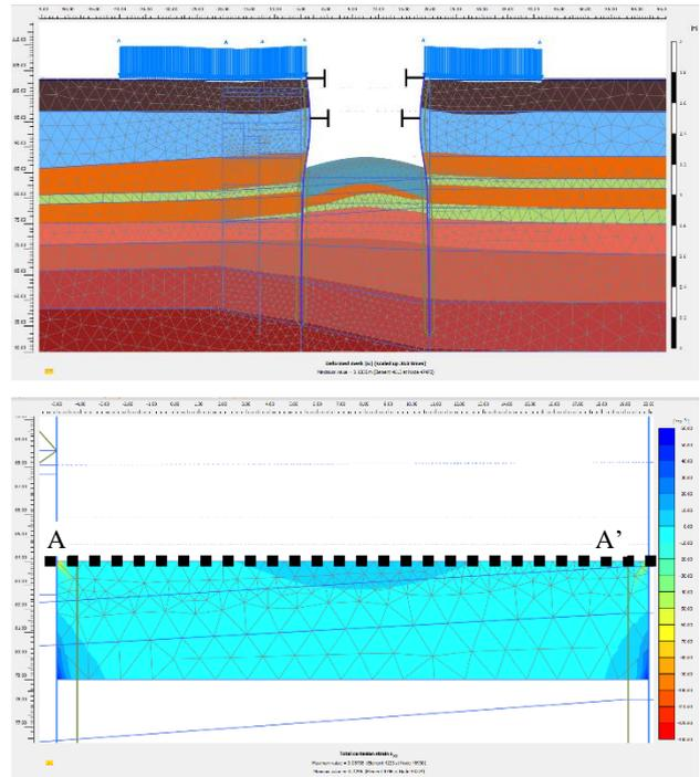
Figure 5 Deformed mesh and horizontal deformations in the ground improvement block during the last stage
