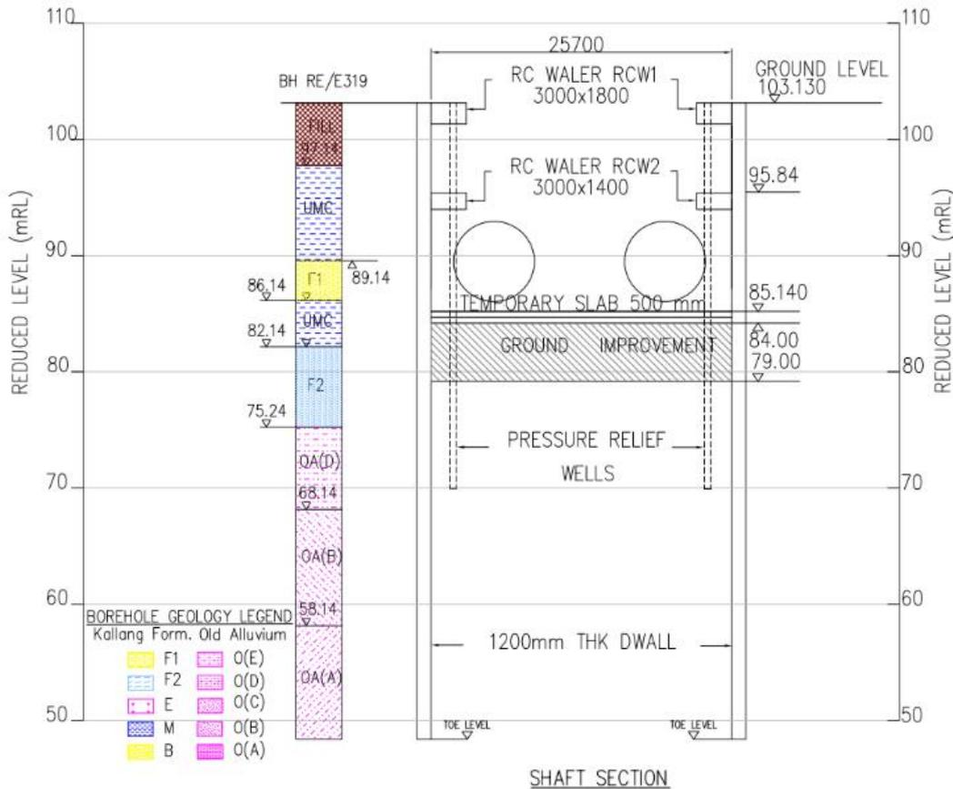
Figure 8 Cross section of the TBM launching shaft with geo profile in the second alternative (use of pressure relief wells)
