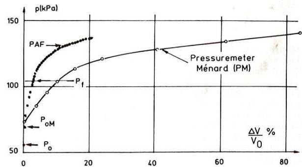
Figure 1 Typical pressuremeter MPM and PAF expansion curves (Baguelin et al. 1978)
