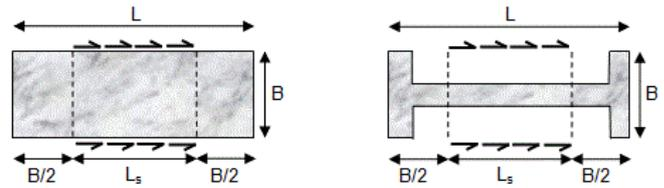
Figure 20 Design lengths for the reaction curves of "barrettes" (MELT, 1993, AFNOR, 2012)
