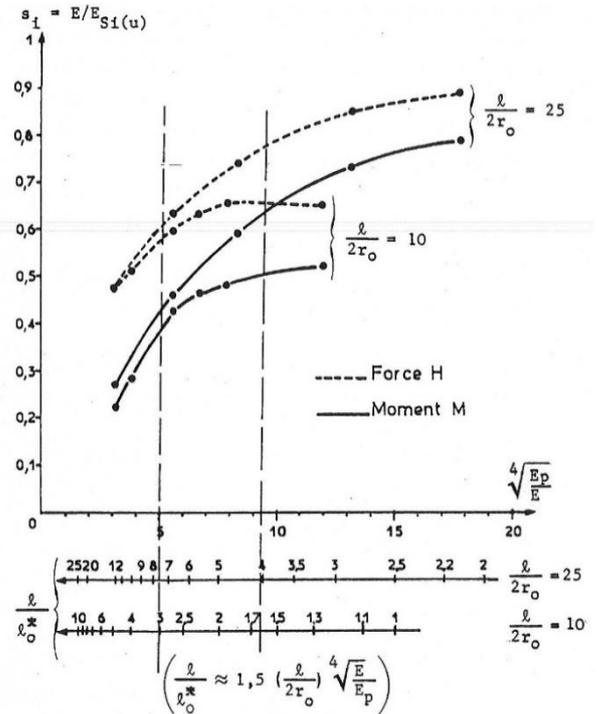
Figure 18 Equivalent horizontal reaction modulus in an intact soil  $E_{s1}(u)$  as a function of the slenderness ratio  $l/2r_0 (= D/2r_0)$ , of the relative pile-soil stiffness  $E_p/E$  and of the head loading (H or M)
