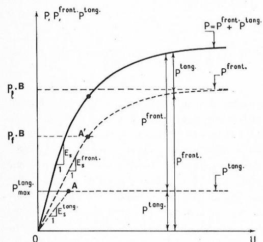
Figure 21 Lateral reaction curves for the design of "barrettes"
