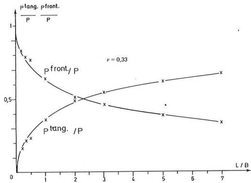
Figure 15  $p^{front.}$  and  $p^{tang.}$  for  $\nu = 0.33$  from 2D finite element calculations
