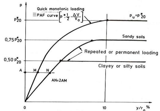
Figure 19  $p$ - $y$  curves derived from PAF expansion curves (Amar et al., 1981)
