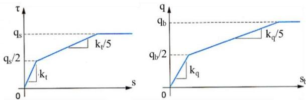
Figure 2 MPM  $\tau$ -s (=t-z) and  $q$ - $s_b$  (=q-z<sub>b</sub>) curves (Frank and Zhao, 1982)
