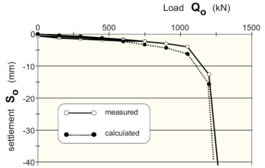
Figure 3 Comparison of measured and calculated load-settlement curves for the Koekelare pile (Bustamante and Frank, 1999)
