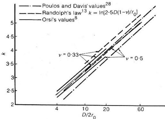
Figure 7 Parameter  $k$  as a function of  $D/2r_0$  and  $\nu$  (in isotropic elasticity) (Baguelin and Frank, 1980)
