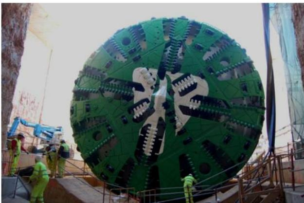
Figure 3 Face of the TBM
