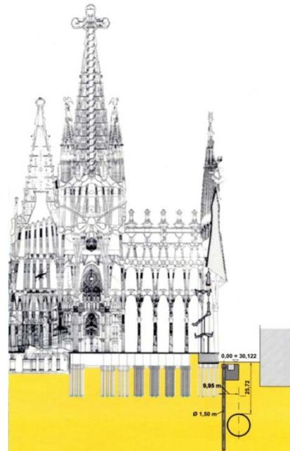
Figure 4 Cross section at Sagrada Familia and AVE tunnel
