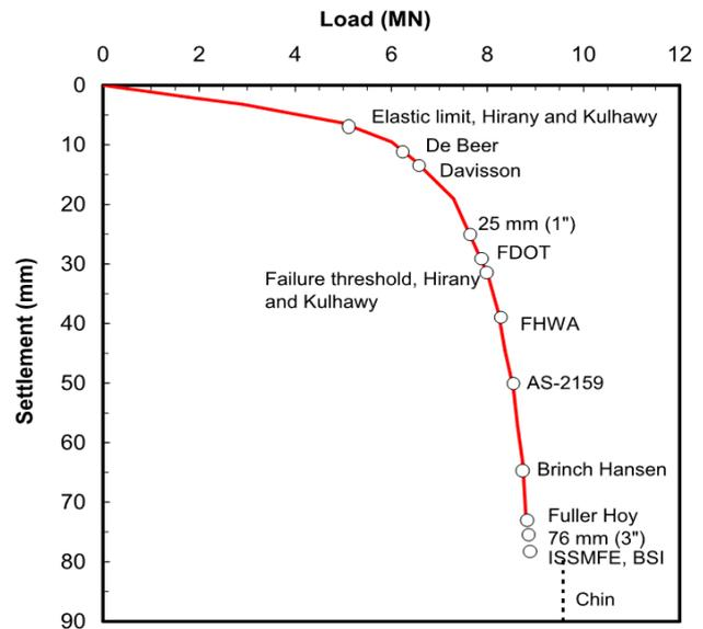
Figure 1 Typical load-settlement curve from a pile-load test in medium dense sand (Zhang and Tang, 2001)
