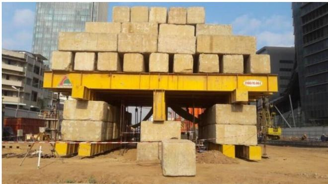
Figure 6 Photograph of static load test with kentledge system (Courtesy of Khmer D&C Technical Consultant, 2018)
