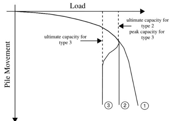
Figure 2 Three types of load settlement curve: 1 – general failure, 2 – punching failure with constant capacity, 3 – punching failure with reduction in the pile capacity
