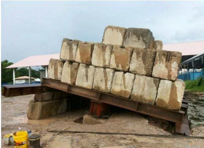
Figure 10 Failure of kentledge system before loading (Courtesy of Profound BV, 2017)
