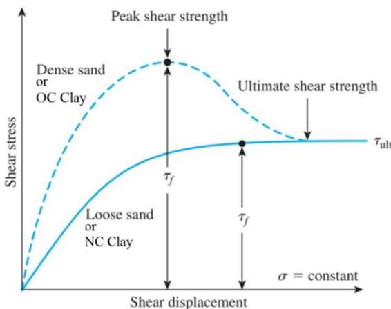
Figure 3 Shear stress versus shear displacement on dense and loose sand (Modified after Das, 2014)
