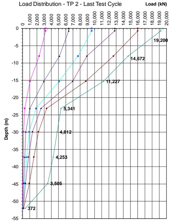
Figure 18 Load distribution curve of test pile no. 2
