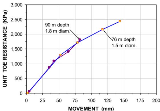
Figure 4 Unit toe resistance measured on a 1.5 and 1.8 m diameter bored pile constructed in silty sandy clay and clayey sand (Fellenius, 2017)
