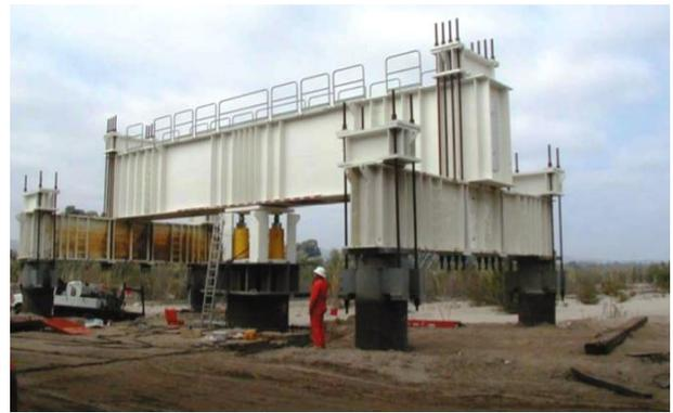
Figure 8 Photograph of static load test with reaction piles (Courtesy of Structville, 2018)
