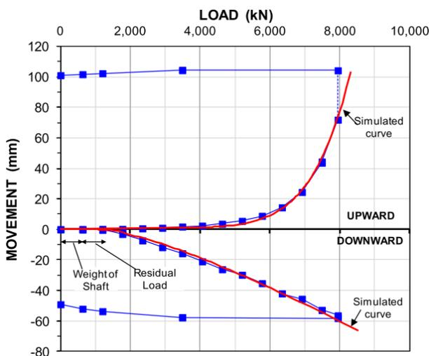
Figure 15 Typical result of a BD-cell test (Fellenius, 2017)
