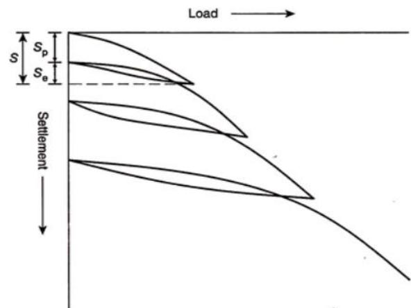
Figure 20 Load-settlement curve in cyclic pile load test (Trishna, 2018)
