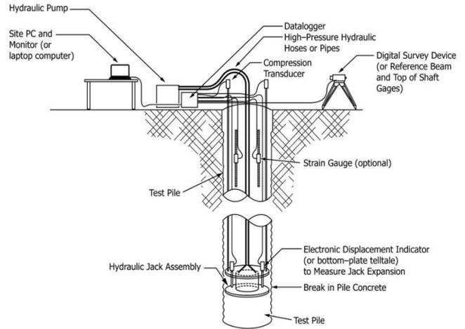
Figure 12 Schematic diagram of a bidirectional test (ASTM, 2018)
