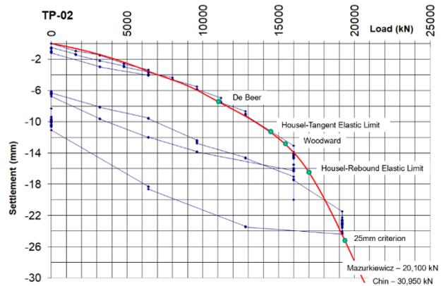
Figure 19 Load settlement curve of TP-01 and TP-02
