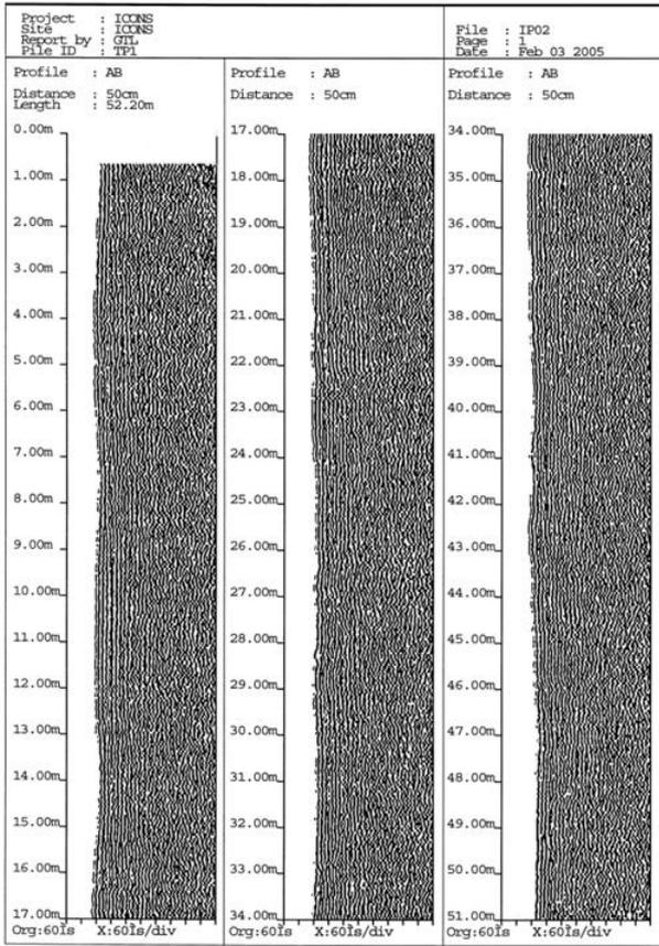
Figure 16 Sonic logging test result show good pile integrity
