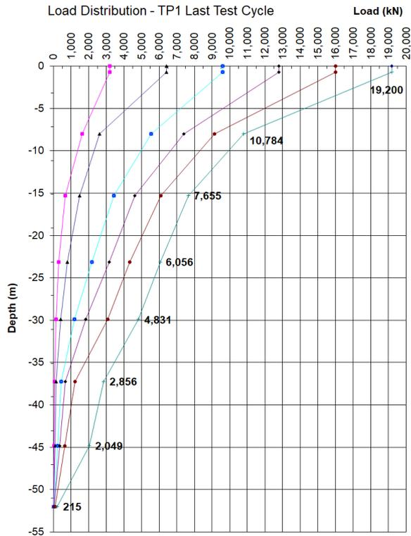
Figure 17 Load distribution curve of test pile no. 1
