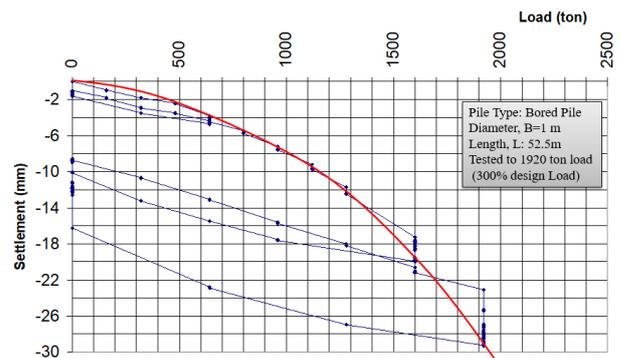
Figure 9 Static loading test result
