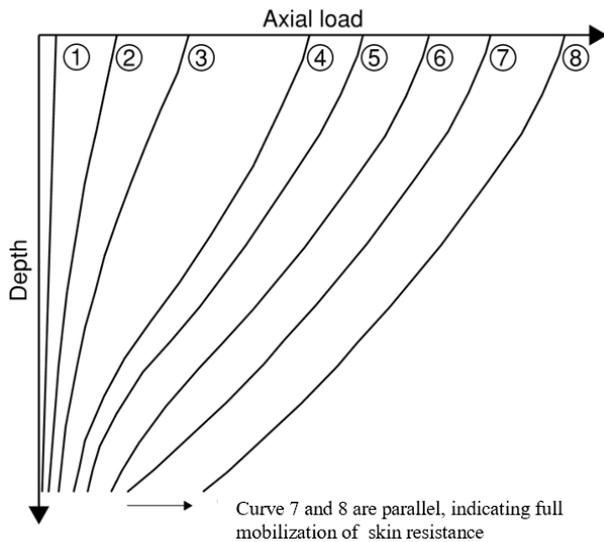
Figure 11 Development of axial load distribution with load steps
