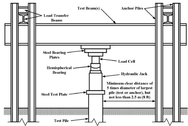
Figure 7 Schematic diagram of a static load test with anchored reaction frame (ASTM D 1143, 2007)
