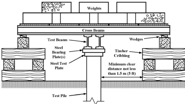
Figure 5 Schematic diagram of static load test with kentledge system (ASTM D 1143, 2007)
