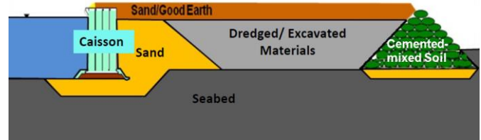
Figure 7 Usage of different reclamation fill materials
