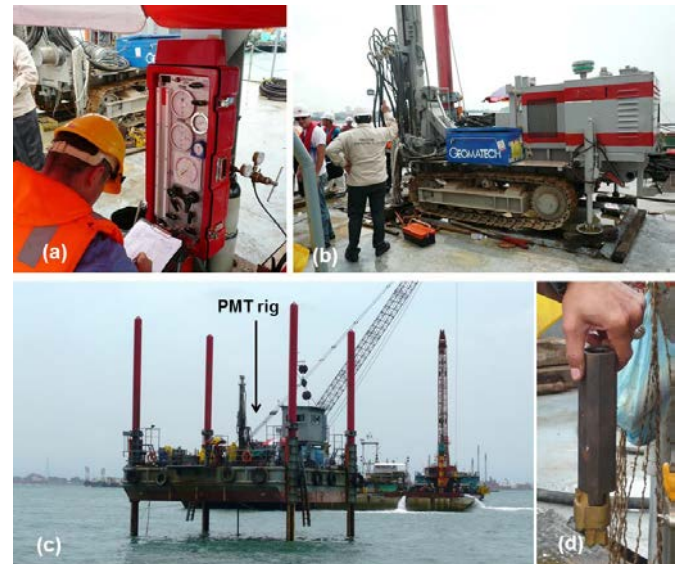
Figure 23 (a) PMT read-out unit; (b) PMT drilling rig; (c) jacked-up pontoon; and (d) STAF drill bit
