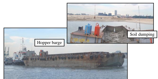
Photo 2 Hopper barge and soil-dumping operation
